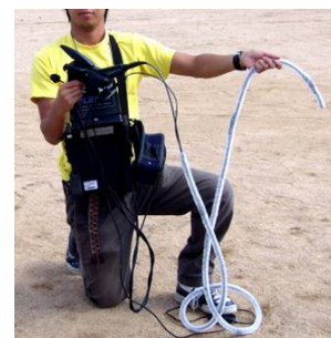
(c) Active Scope Camera (Tohoku University)
