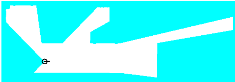
(c) Using this point, a flood fill algorithm is used to fill the polygon with free space.
