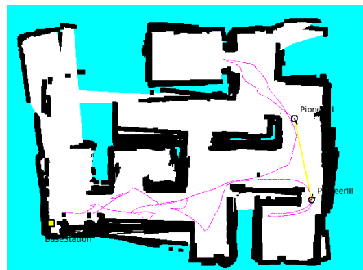
(f) PioneerIII returns to rendezvous to give PioneerII a second chance. Pioneers II and III meet, and exploration can proceed as normal.
