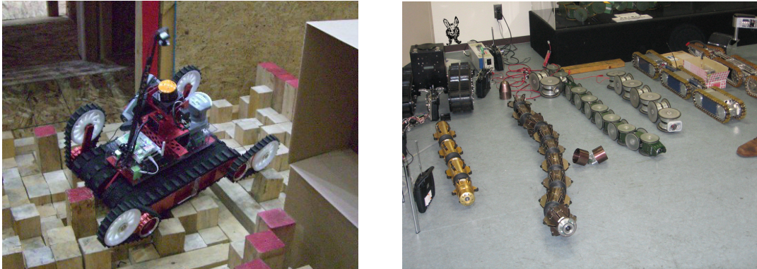
Figure 2.5: Recent rescue robot designs. The Kenaf robot (left), developed in part at the University of Tohoku, Japan, has two main tracks and four tracked “flippers” which allow it to climb stairs and traverse difficult terrain. At Prof. Matsuno’s laboratory in Osaka University, there is a strong focus on snake-like robots that are becoming ever smaller and more mobile (right).
