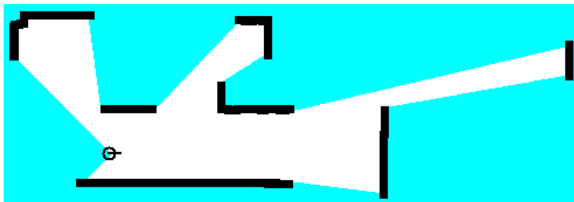
(d) Scan points sufficiently close together are connected as obstacles.
