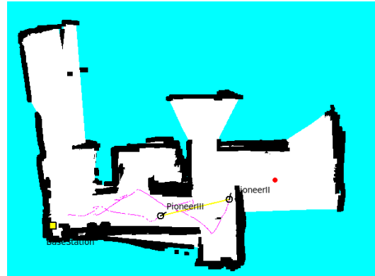
(b) After some time, PioneerIII must return to BaseStation. PioneerII chooses the red point as a rendezvous location.
