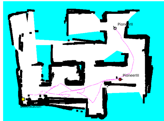
(d) Some time later, PioneerIII reaches the rendezvous point. PioneerII has mistimed rendezvous, and is still exploring.
