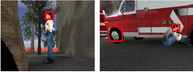
Fig. 1. Our face detector can recognise faces at greater distances than the VictimSensor. Some detections are false positives, but these can be used as negative examples in subsequent levels of training.
